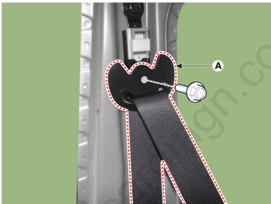
3. Disconnect the front seat belt retractor connector (A).
