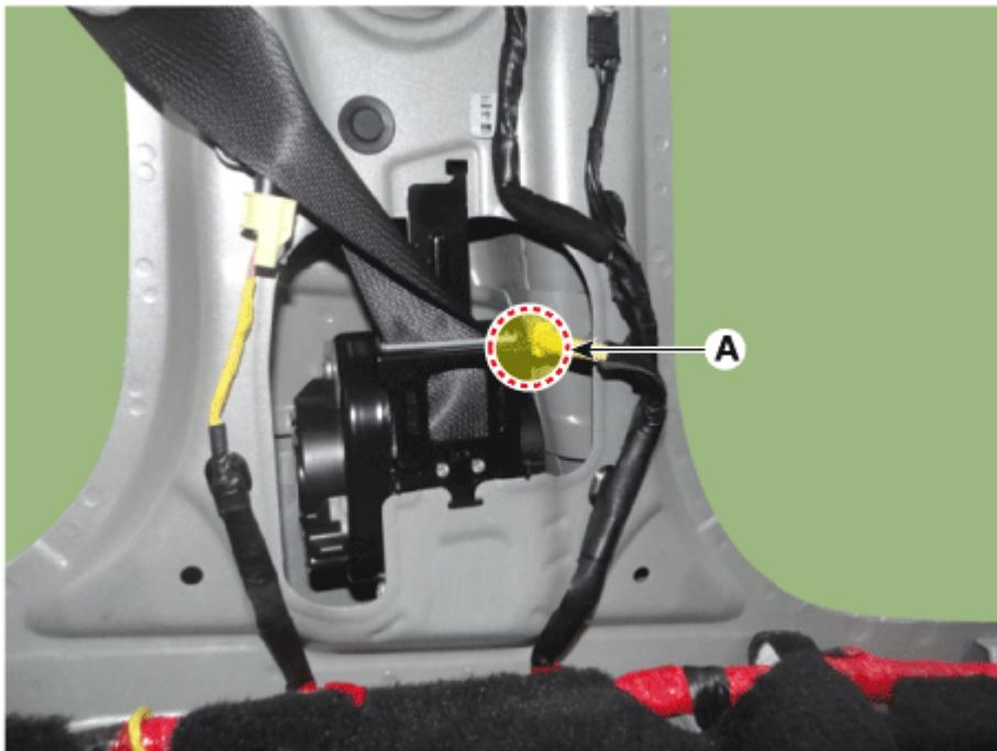
4. Remove the front seat belt retractor (A) after loosening the mounting bolt.
